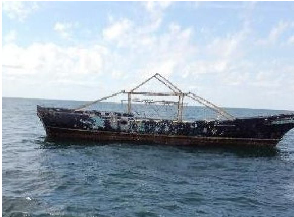
To add vertical relief to a 53-foot concrete hulled boat, steel framing was welded to the deck.
